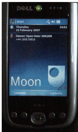
Figure 1. The opening screen of the PDA. The buttons below the screen can be used to launch programs.
