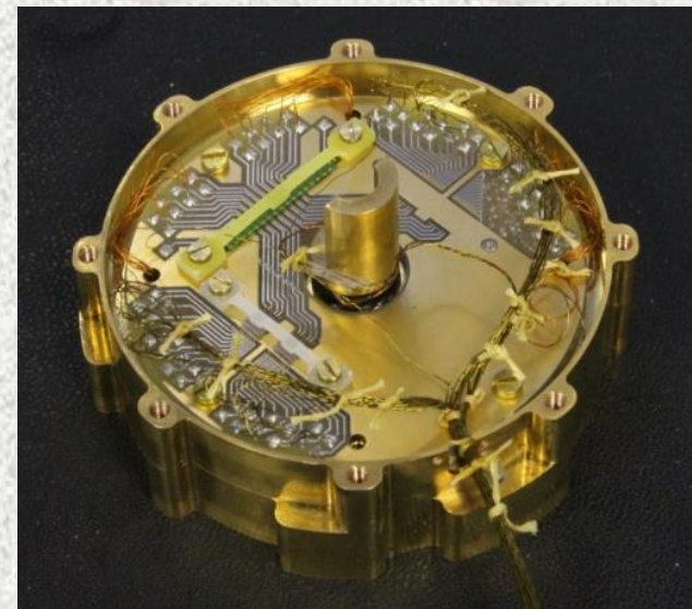
Small-format 16 element test arrays with integrated optical backshorts Few-mode, 10-20, lightpipe coupling (developed fabrication technology for S and L Band)
