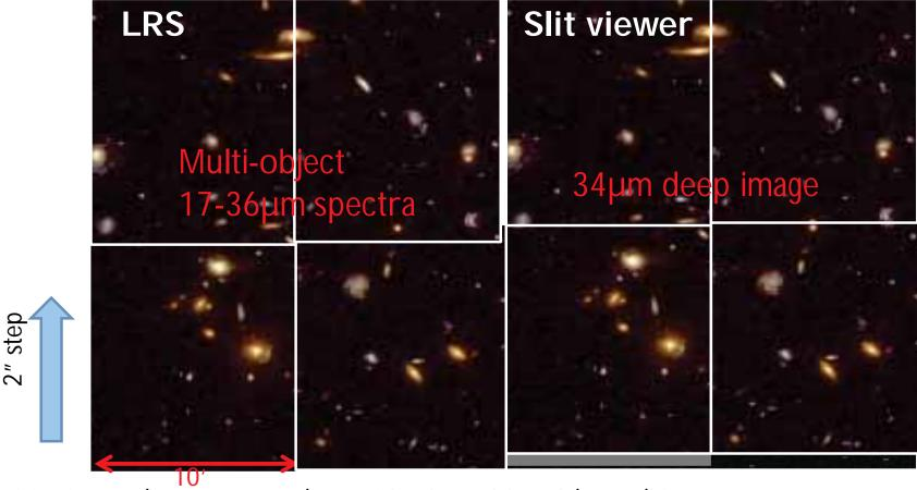
Slit viewer (10' x 10' FoV) provides broad-band (R = 5) images at  $\lambda_c$  = 34µm
