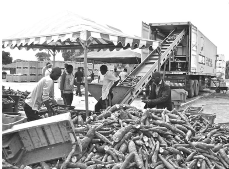
Cassava being loaded into the Dadtco processing machine, which fits into a 40 foot container.
