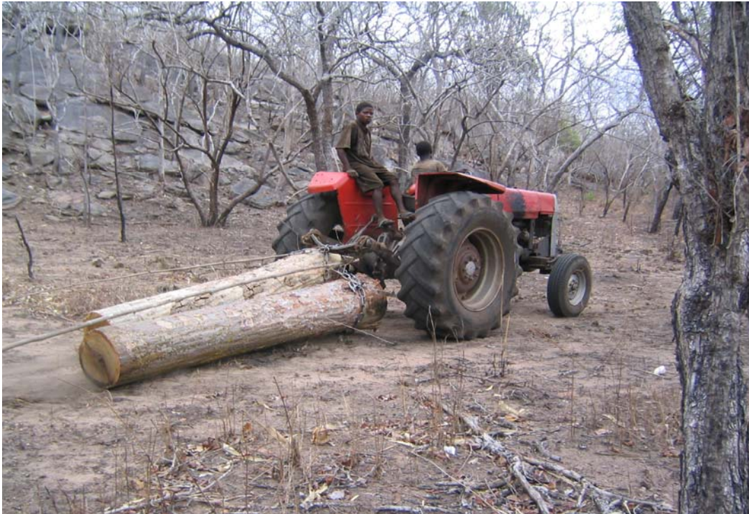
Photo 4: Extraction of logs using an agricultural tractor (photo courtesy R Lautelienan).
